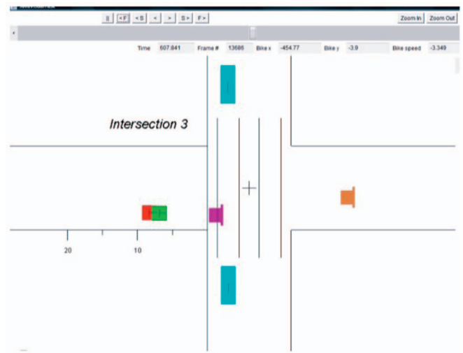
Fig. 5. A screenshot of the automatic data coding and after-action review tool. The visualization shows an abstract top-down view of the automatically coded rider's stopping position (red square), starting position (green square), the rider (pink square), and the peer waiting for on other side of the intersection (brown square). The front and back vehicles of the gap chosen by the rider are represented as blue rectangles in the crossing street.
