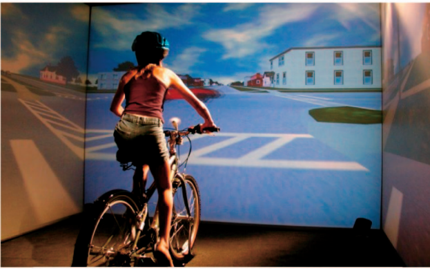
Fig. 1. Immersive bicycling simulator.
