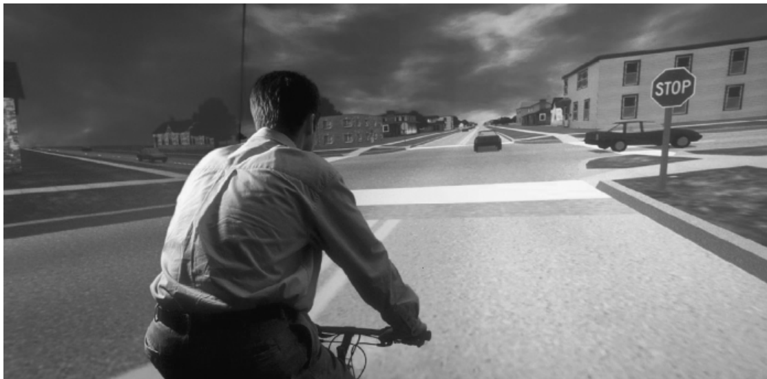
Figure 1. Photograph of an adult riding an instrumented bicycle through the virtual environment. (Note that there was no traffic on the street with participants in our experiment.)
