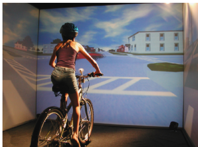
Fig. 1. The bicycling simulator. Note that the visual angles are correct from the viewpoint of the rider.
