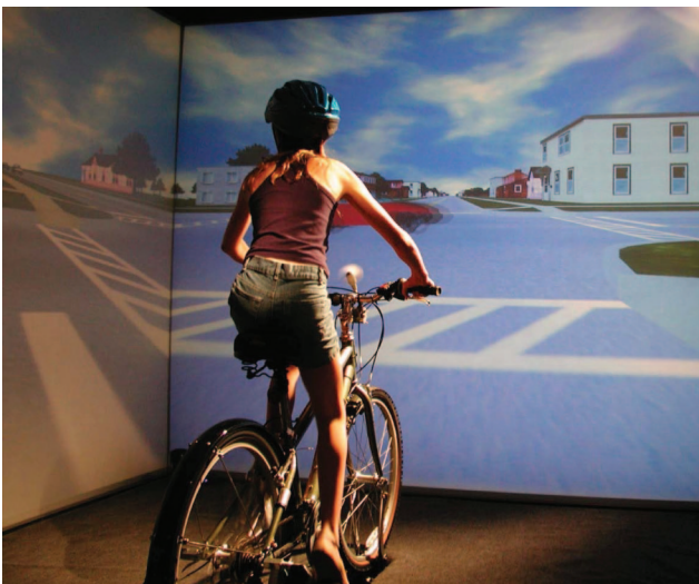
Figure 2. Photograph of the bicycling simulator. Note that the visual angles are correct from the viewpoint of the rider.
